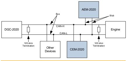
Figure 1 - AEM-2020 and CEM-2020 CAN Bus Interface
